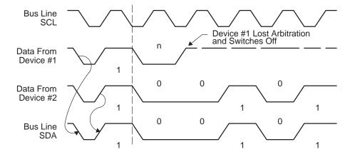
If the arbitration procedure is in progress when a repeated START condition or STOP condition is transmitted on SDA, the master transmitters involved in arbitration must send the repeated START condition or STOP condition at the same position in the format frame. Arbitration is not allowed between:
